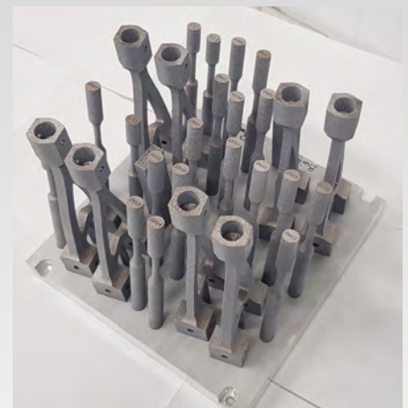
Figure 12 Wishbone and specimens for validation testing
