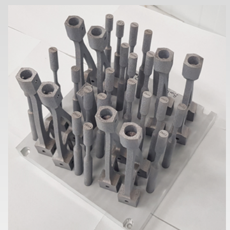
Figure 12 Wishbone and specimens for validation testing
