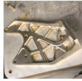
Bracket before separation from build plate
