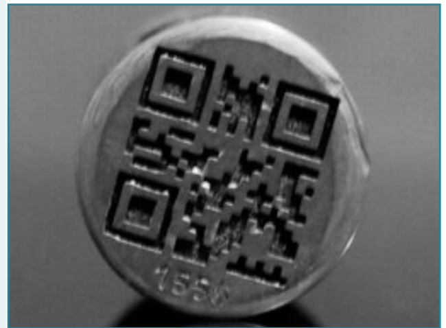
Enhanced material identification through using embedded QR codes - 3D printed part with QR code by MolyWorks (Image courtesy of MolyWorks) 10
