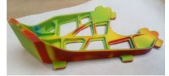
Polymer bracket colour-mapped showing predicted distortion
