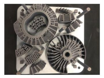
Build bed configuration showing fin geometries
