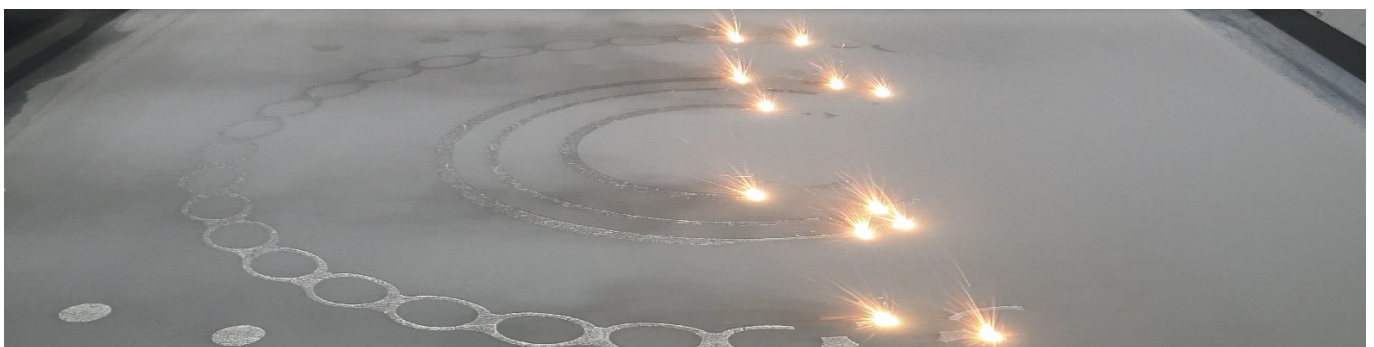
Figure 13: An example of laser scanning strategy of 12 beams on a multi-laser system [SLM Solutions NXG XII 600]. Image courtesy of SLM Solutions.
