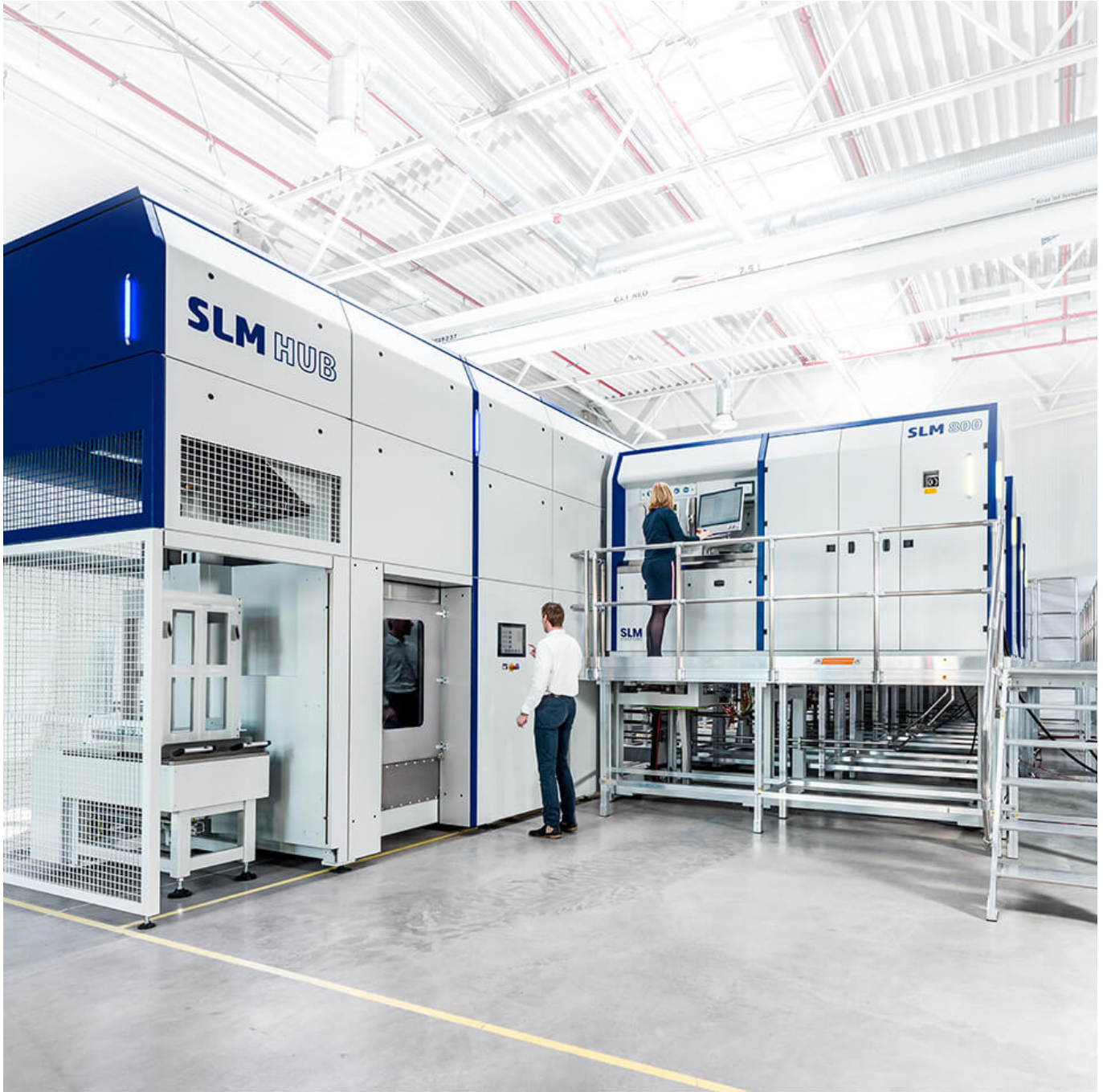
Figure 11: SLM Hub is an automated powder handling station. With automated transport of build cylinders with dedicated locations for pre-heating and cooling. Other features include depowdering and a centralised powder supply. Image courtesy of SLM Solutions.
