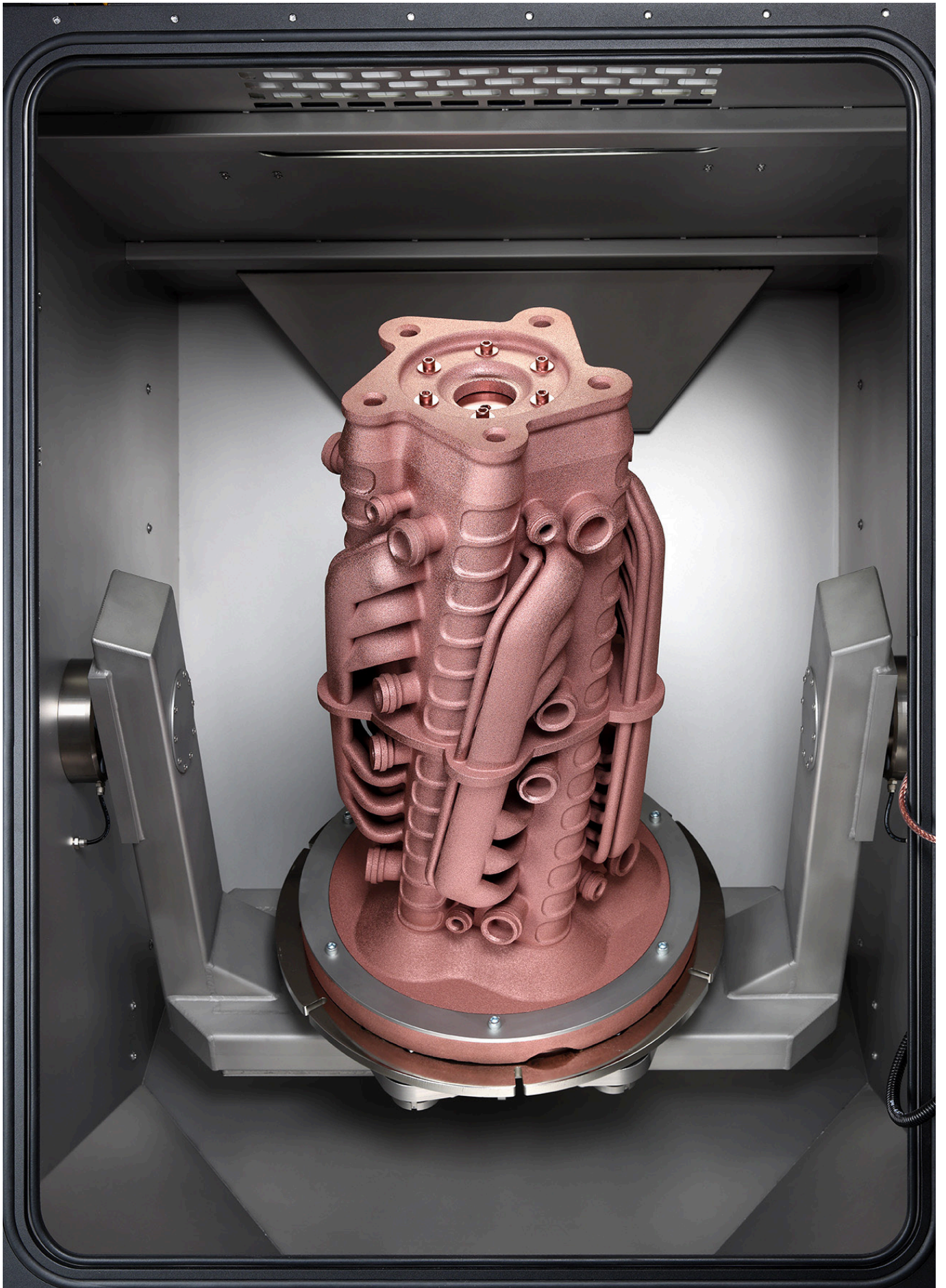
Figure 14: Large AM part installed in a Solukon depowdering system SFM-AT1000-S. Image courtesy of Solukon.
