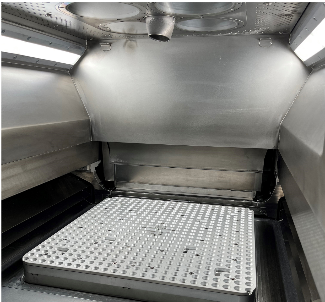
Figure 12: EOSYSTEM SmartCal calibration plate being installed on MTC's EOS M400-4. Image courtesy of The MTC.
