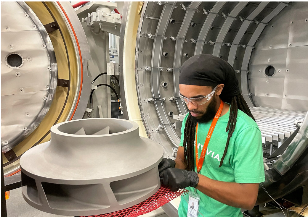
Figure 4: Impellor component produced on SLM Solutions NXG XII 600. Dimension: ~Ø550 mm x 300 mm Z-height. Build Time:~7 days. Material: Nickel Superalloy. Courtesy of Sintavia.
