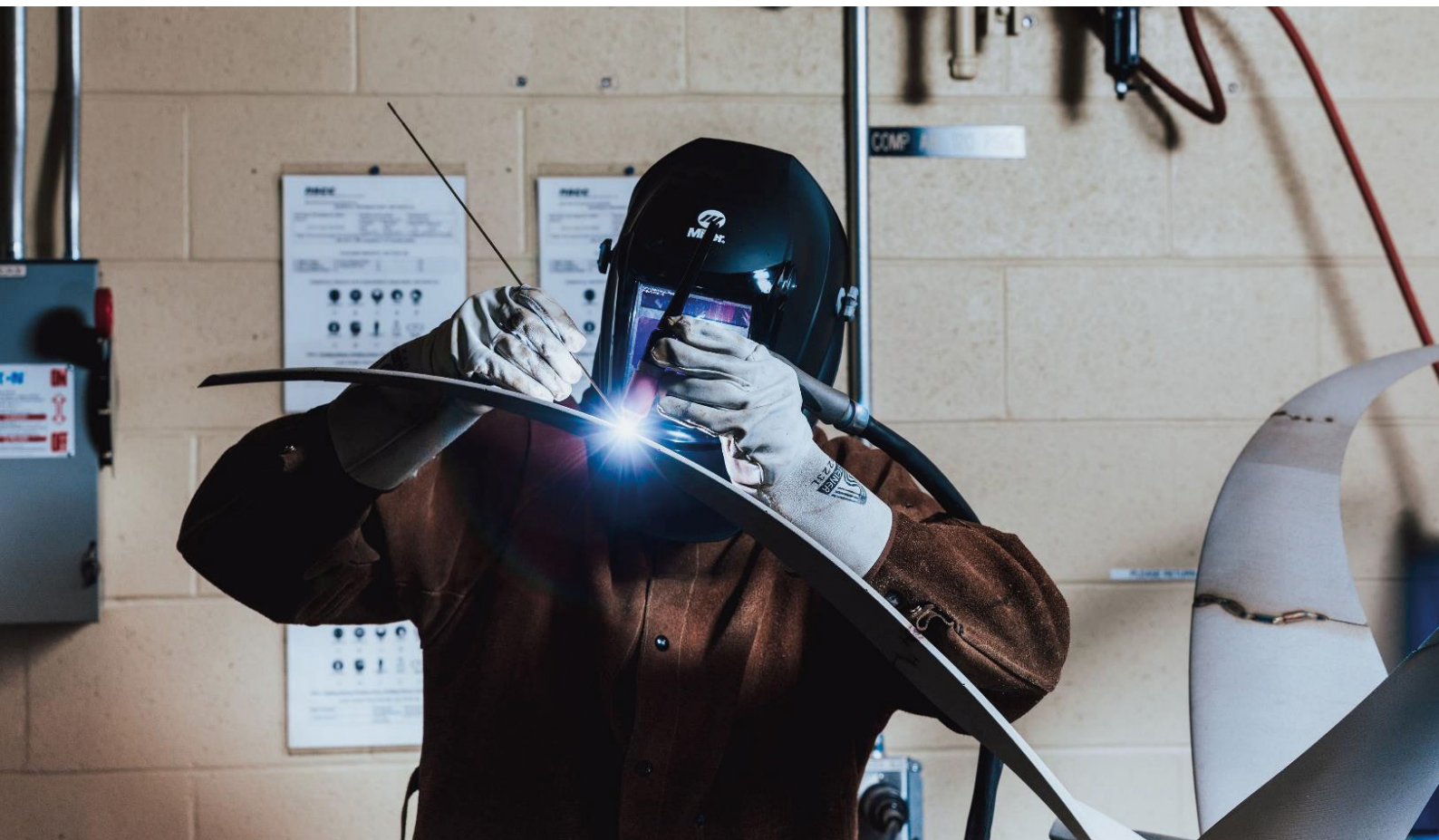
Figure 2 Welding together tidal turbines sections produced using PBF-LB. Courtesy of Biome Renewables/Nova Scotia Community College.
