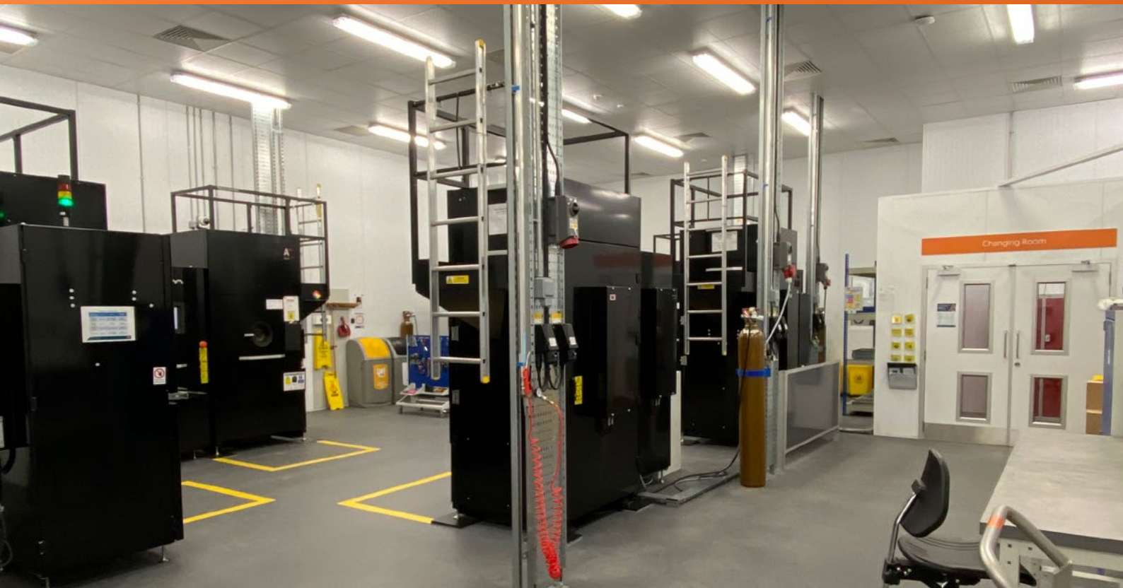
AM build processing room, housing six Arcam EBM machines
